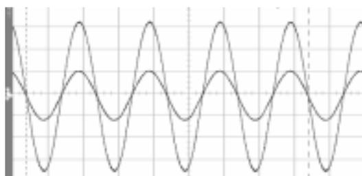
Diagram 7: Input voltage and current waveform
